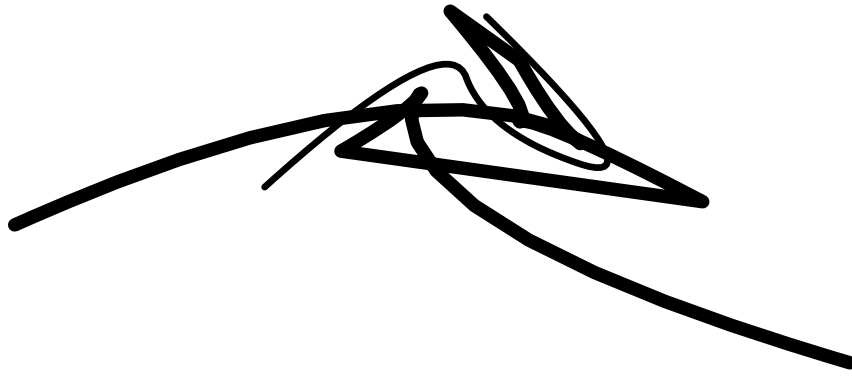
Figure 27: The evolute (thick) of a freeform curve (thin) can be computed using EVOLUTE.
