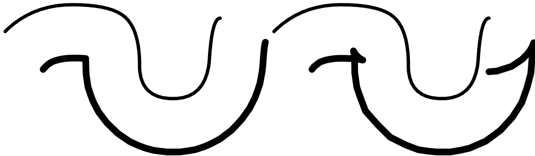
Figure 3: Adaptive offset approximation (thick) of a B-spline curve (thin). On the left, the self intersections in the offset computed in the right are eliminated. Both offsets were computed using AOFFSET. (See also Figure 31.)
